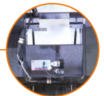
Patient information inserts are automatically printed, indexed, verified, folded and inserted with the integrated Continuous Print System
